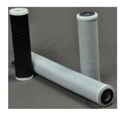
Activated carbon block type cartridge is made from coconut-shell. Activated carbon is molded together with synthetic fiber binder via a wet production method. Activated Carbon block cartridge is well suited for removal of organic tastes, odors, chlorine & sediments. They are ideal for filtration of potable water. Cartridges are made from FDA approved materials.
