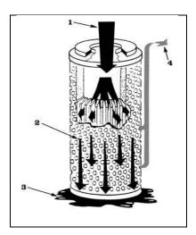
Coalescing filter cartridges are especially designed for moisture, oil & particulate removal from air and gases. The cartridge has stainless steel shell and support components. Stainless steel outer core supports the filter media since the flow differential pressure is from inside to outside. The cartridge is made from HEPA filter media which in gas service will remove better than 0.3 micron particles. HEPA filter media is supported by SS wire mesh to take care of high pressure differentials.
