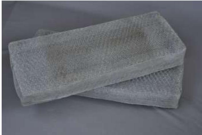
Demister pads or Mist eliminators are porous blankets of metal wire or plastic knitted mesh, designed and constructed for the efficient, economical removal of entrained liquid droplets from vapor streams. Demister Pads can be fabricated in any required size and shape and may be installed in new or existing process vessels.
