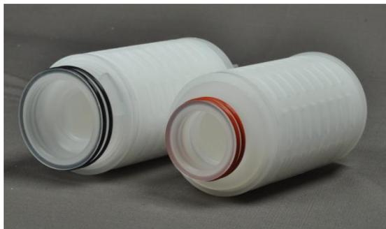
Polyethersulfone (PES) absolute rated membrane cartridges are inherently hydrophilic and contain no added surfactants or wetting agents that could alter the taste in beer, wine, bottle water & other beverages. PES absolute filters are sterile filters offering superior flow characteristics, high contaminant holding capacity and consistent removal of particles and micro organisms. The cartridges are 100% integrity tested to assure reliability.
