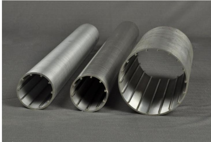
Welded wedge wire products are the most reliable, long lasting and maintenance free filter media. It consists of V shaped wire which is welded on to support rods. The 'V' shaped wire while welding to the support rod is controlled very accurately, as it forms the slot through which the filtrate flows. These welded wedge wire products which can be in the form of tube or rectangular pieces can replace conventional media like wire mesh cloth.
