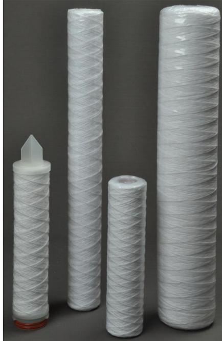
SS Filters Wound Filter Cartridges are manufactured using a high speed, continuous wind process which creates a superior one-piece filter with hundreds of diamond shaped tunnels that get progressively smaller from the outer diameter to the core. Finer particles are progressively trapped as fluid travels to the centre of the filter allowing for much greater retention capacity than straight surface filter media of same dimensions & porosity.
